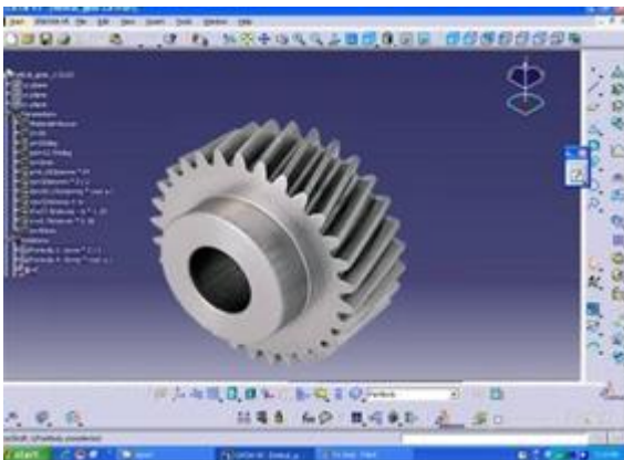
Figure 2. Model of helical gear generated by CATIA5
