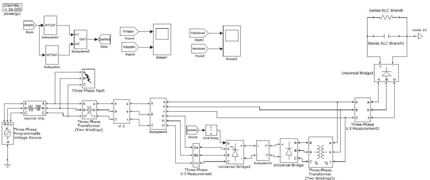
Fig 4.5 Simulink diagram for mitigation of voltage dip using DVR for linear load
