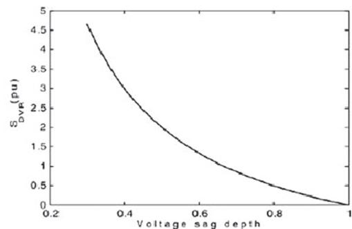
Fig 4.3 Sdvr vs Voltage Sag Depth
