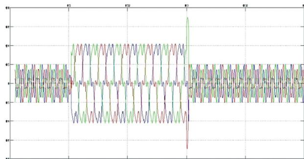
Fig 5.1.3 Three phase DVR voltage
