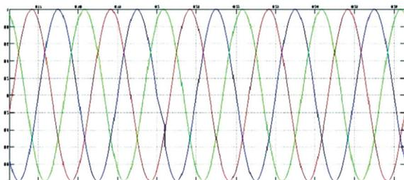
Fig 5.4.2 Three Phase Load Voltage
