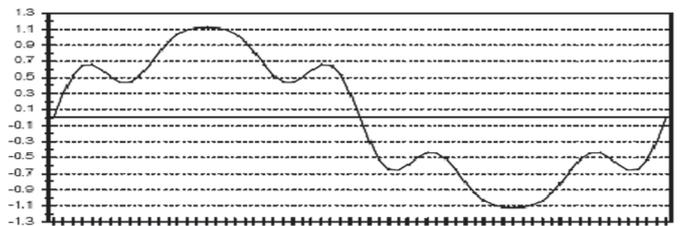
Fig 2.2 Fundamental with two harmonics
