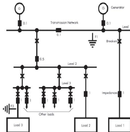
Fig. 2.1 The cause of voltage dips
