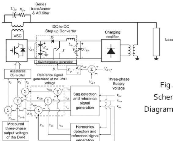
Fig 4.2 Schematic Diagram of DVR
