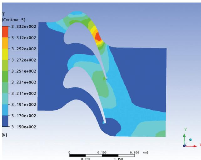
Fig 4.1.3 Case 2 Temperature contour at mid span for T=3150K
