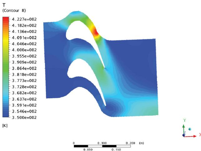
Fig 4.1.3 Case 1 Temperature contour at mid span for T=3500K
