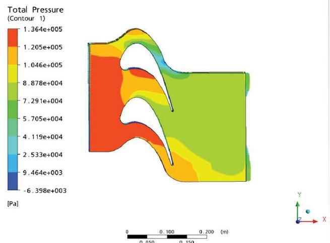
Fig. 4.1.2 case1 Total Pressure contours at mid span for T=3500K
