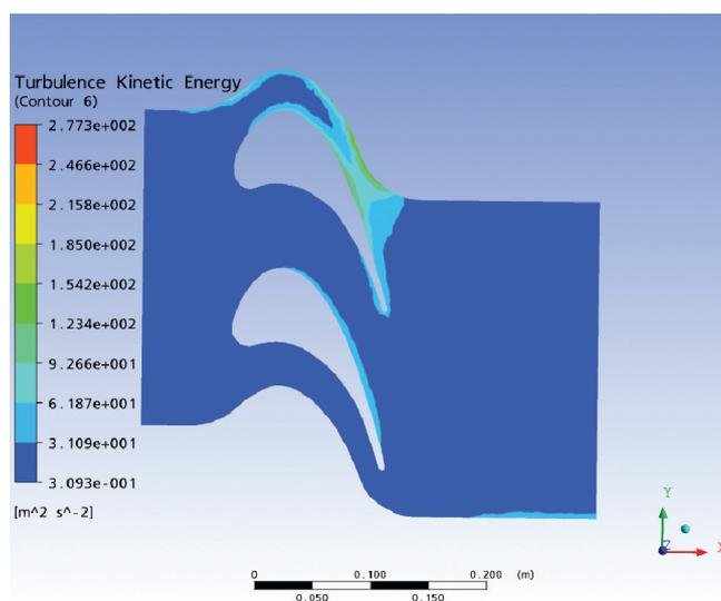
Fig 4.1.6 Case 2 Turbulence Kinetic Energy at mid span for T=3150K
