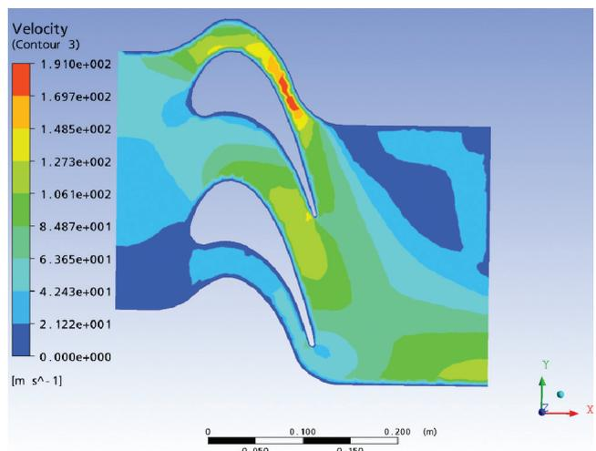
Fig 4.1.4 Case 2 Velocity contour at mid span for T=3150K
