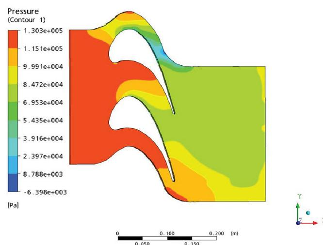
Fig. 3.1.1 Case1 Pressure contours at mid span for T=3500K
