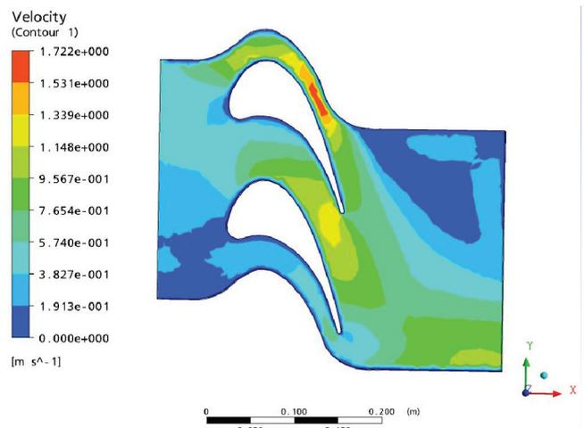
Fig 4.1.4 Case 1 Velocity contour at mid span for T=3500K
