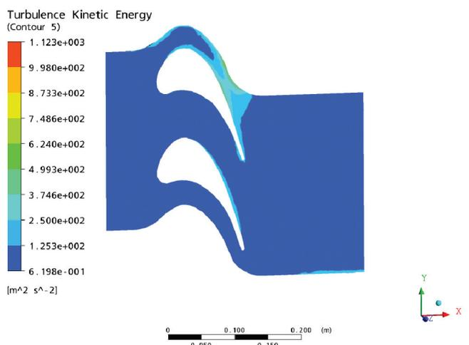
Fig 4.1.6 Case 1 Turbulence Kinetic Energy at mid span for T=3150K
