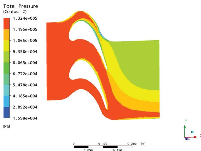
Fig. 4.1.2 case2 Total Pressure contours at mid span for T=3150K
