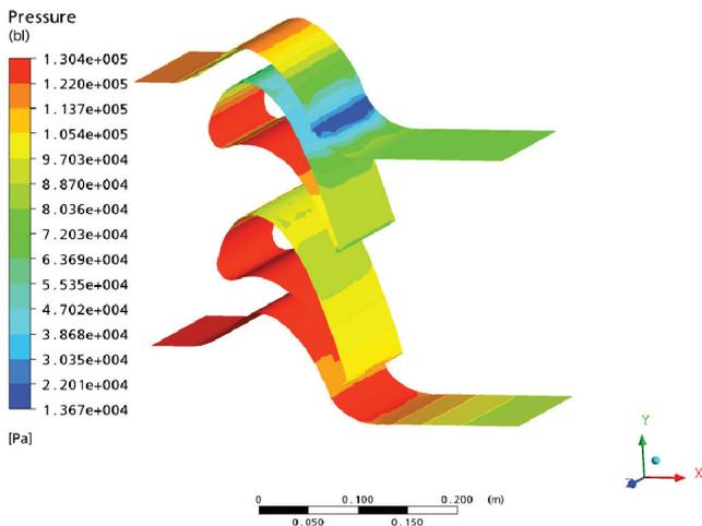
Fig.3.1.1 case1 Pressure contours at Blade side View at T=3500K
