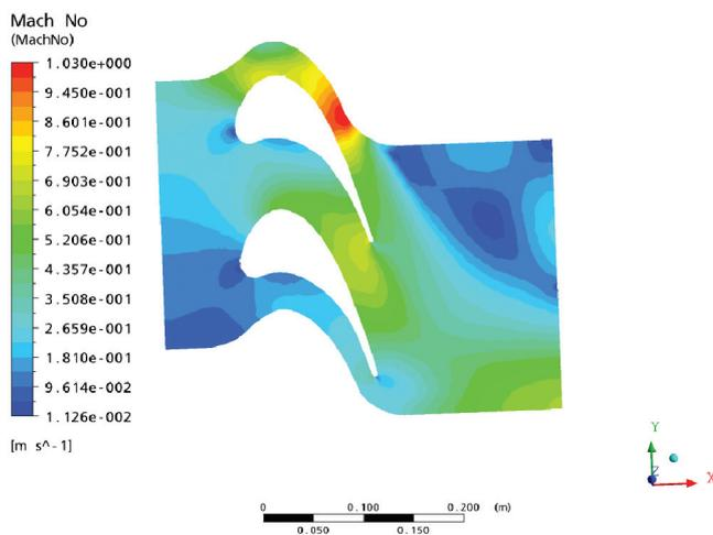
Fig 4.1.5 Case 1 Mach Number Distribution at mid span for T=3500K
