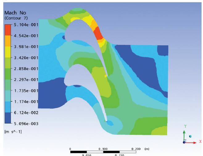
Fig 4.1.5 Case 2 Mach Number Distribution at mid span for T=3150K
