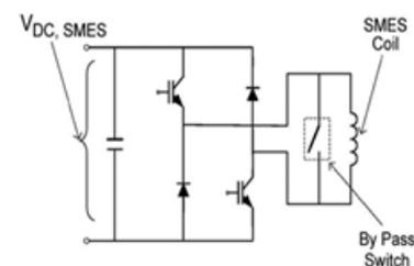
**Fig3.1 Class-D dc-dc chopper using an SMES coil**
