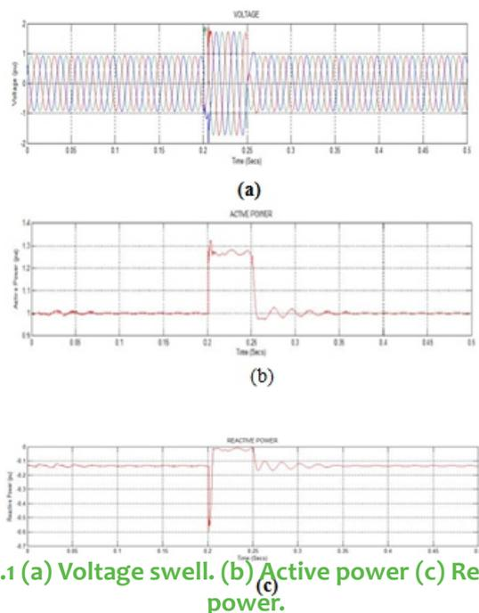
Fig.4.1 (a) Voltage swell. (b) Active power (c) Reactive power.
