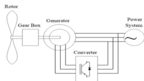
**Fig1.1: Principle of a DFIG connected to wind turbine**
