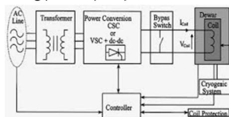
Fig2.2 Schematic diagram of SMES Connected to grid
