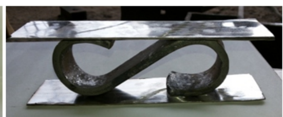
Welded steel sandwich composite structure
