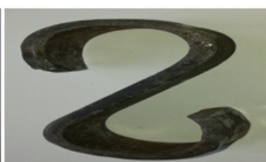
Fig Stainless steel face and mild steel core
