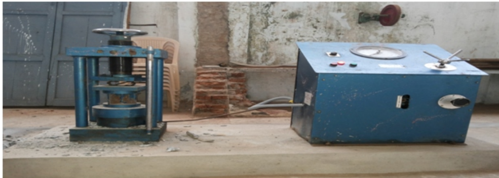
compression testing on CTM machine
