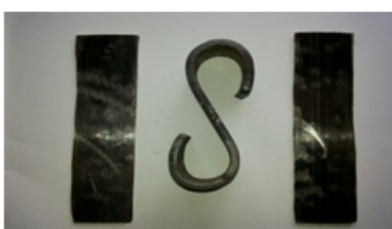
Fig Stainless steel face and mild steel core
