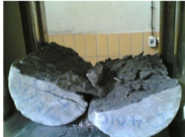
Control concrete after test
