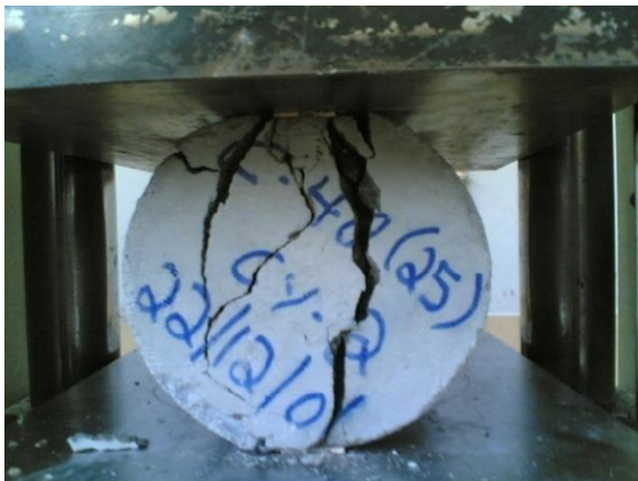
Rubberized concrete at failure
