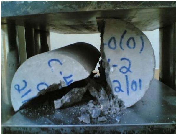
Control concrete at failure
