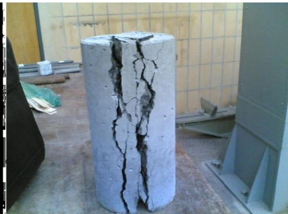
Rubberized concrete after test
