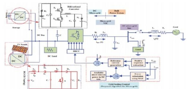
Figure 1: Hybrid Energy Conversion System under Consideration
