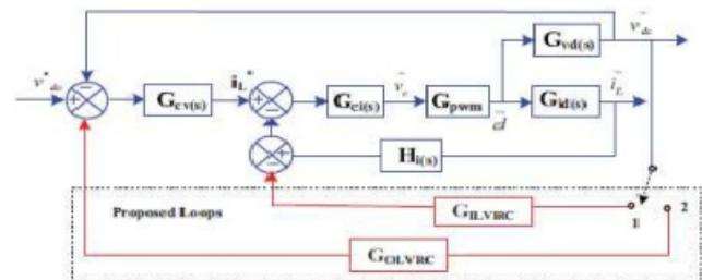
Figure 4: Inner and Outer Loops of Battery Converter with MACMC
