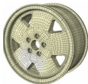
Meshed geometry of Wheel rim
