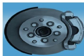
**Figure 1: Disc Brake full assemble view**
