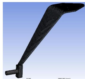
**Figure 2.2: 3D-meshed model of landing gear's leg**
