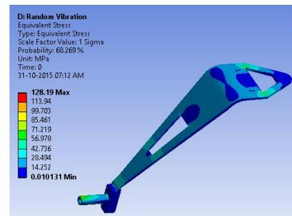
**Figure 5.2: Von-mises stress plot for spectrum analysis**
