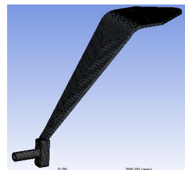
Figure 2.2: 3D-meshed model of landing gear's leg
