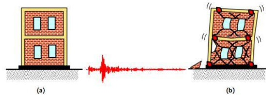
Figure 1.3 : Earthquake-resistant and NOT Earthquake-Proof :Damage is expected during an earthquake in normal constructions (a) undamaged building, and (b) damaged building.
