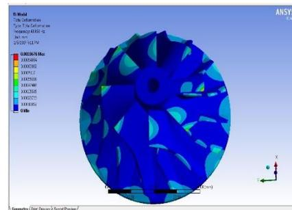
Mode shape 4 of aluminum alloy. At this mode the natural frequency of the impeller is 43.058Hz and deformation is 0.0010676 mm.
