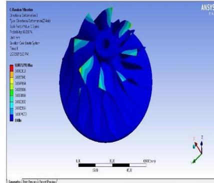
Deformation of the Magnesium Alloy Impeller in Z direction in random vibrational analysis. The deformation value is 0.0071795 mm.
