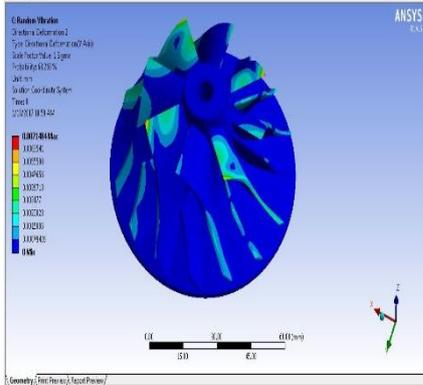
Deformation of the Monel K500 Impeller in Y direction in random vibrational analysis. The deformation value is 0.007148 mm.
