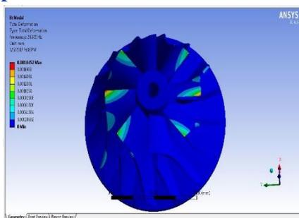
Mode shape 1 of aluminum alloy. At this mode the natural frequency of the impeller is 24.535Hz and deformation is 0.0018452 mm.
