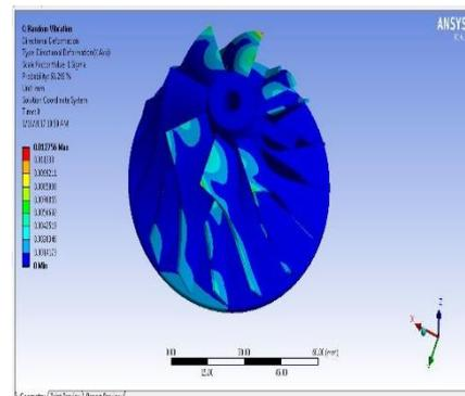
Deformation of the Monel K500 Impeller in X direction in random vibrational analysis. The deformation value is 0.0012756 mm.
