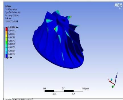
Mode shape 1 of Monel K500. At this mode the natural frequency of the impeller is 22.881Hz and deformation is 0.0010518 mm.
