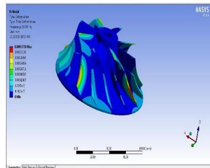
Mode shape 2 of Monel K500. At this mode the natural frequency of the impeller is 26.587Hz and deformation is 0.0003728 mm.
