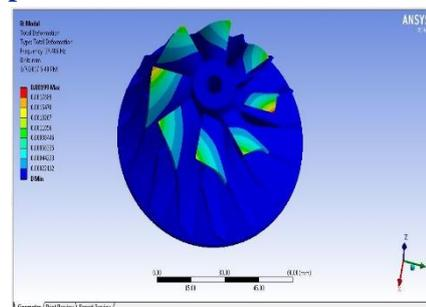
Mode shape 1 of Magnesium Alloy. At this mode the natural frequency of the impeller is 37.486Hz and deformation is 0.00199 mm.
