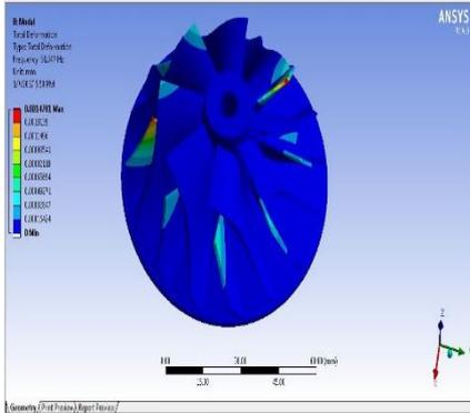
Mode shape 2 of Magnesium Alloy. At this mode the natural frequency of the impeller is 51.047Hz and deformation is 0.0014781 mm.
