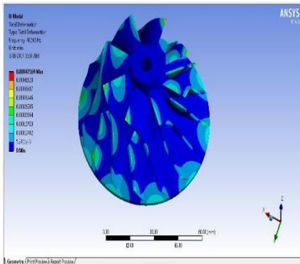
Mode shape 4 of Monel K500. At this mode the natural frequency of the impeller is 40.565Hz and deformation is 0.00047169 mm.
