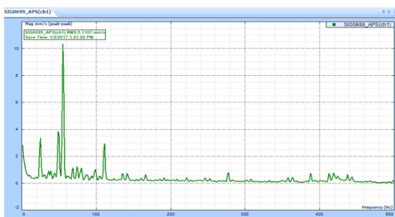
Frequency spectrum at top of the Impeller
