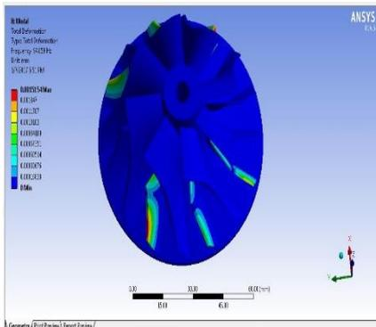
Mode shape 4 of Magnesium Alloy. At this mode the natural frequency of the impeller is 94.059Hz and deformation is 0.0015154 mm.
