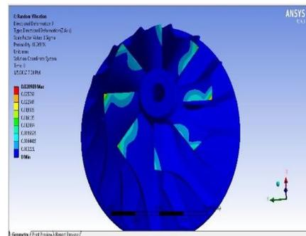
Deformation of the Aluminum Alloy Impeller in Z direction in random vibrational analysis. The deformation value is 0.028989 mm.
