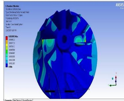
Deformation of the Aluminum Alloy Impeller in X direction in random vibrational analysis. The deformation value is 0.010892.
