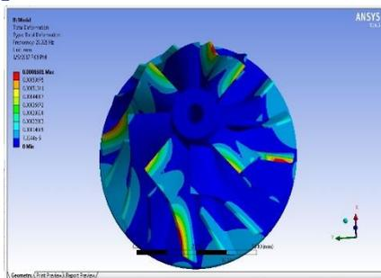
Mode shape 2 of aluminum alloy. At this mode the natural frequency of the impeller is 28.329Hz and deformation is 0.0006601 mm.
