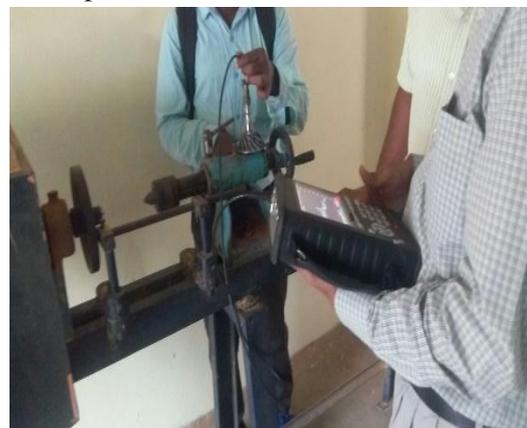
Vibration measurement at the top of the Impeller using FFT analyzer and piezo electric sensor
