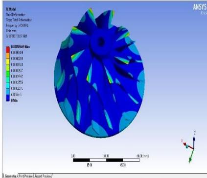
Mode shape 3 of Monel K500. At this mode the natural frequency of the impeller is 34.568Hz and deformation is 0.00055669 mm.
