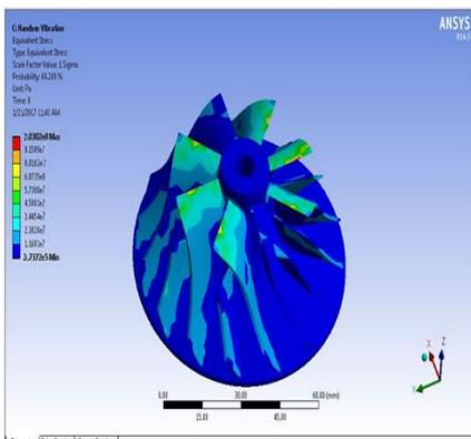
Stress induced in Monel K500 Impeller in random vibrational analysis. The stress induced is 203.02 MPa
