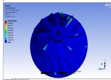
Mode shape 5 of aluminum alloy. At this mode the natural frequency of the impeller is 48.043Hz and deformation is 0.0048178 mm.
