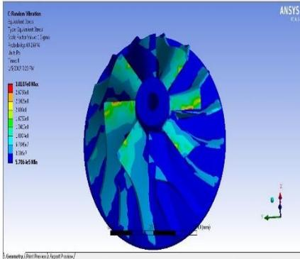
Stress induced in Aluminum Alloy Impeller in random vibrational analysis. The stress induced is 301.07 MPa
