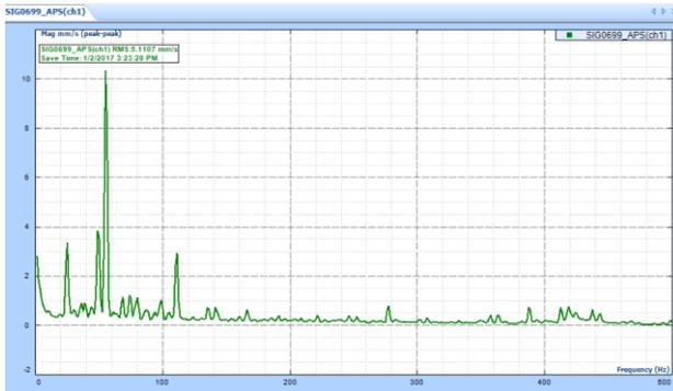
**Frequency spectrum of the impeller**
