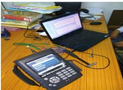
Photograph of instruments, hardware and software used for Natural Frequency Test (NFT) on Impeller
