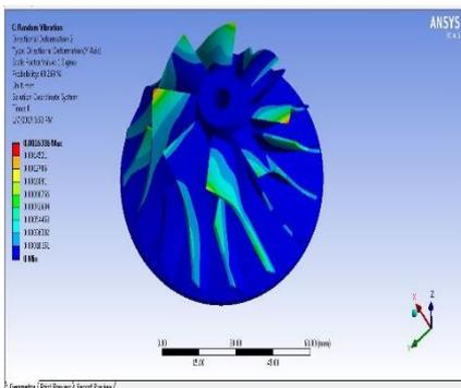
Deformation of the Magnesium Alloy Impeller in Y direction in random vibrational analysis. The deformation value is 0.006336 mm.
