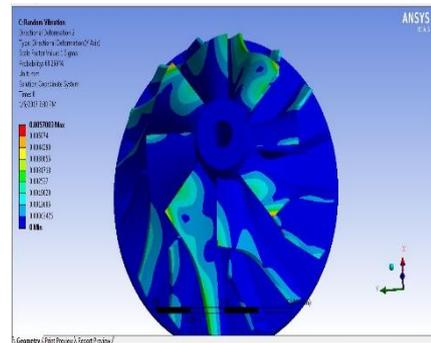
Deformation of the Aluminum Alloy Impeller in Y direction in random vibrational analysis. The deformation value is 0.0057083 mm.
