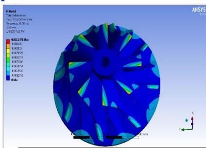
Mode shape 3 of aluminum alloy. At this mode the natural frequency of the impeller is 36.7555Hz and deformation is 0.0011476 mm.
