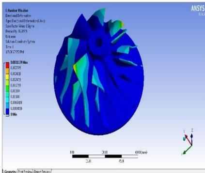
Deformation of the Magnesium Alloy Impeller in X direction in random vibrational analysis. The deformation value is 0.0031139 mm.
