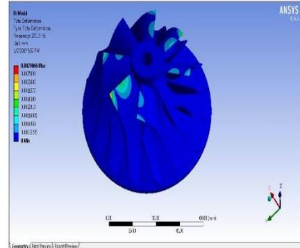
Mode shape 5 of Magnesium Alloy. At this mode the natural frequency of the impeller is 127.15Hz and deformation is 0.0029066 mm.
