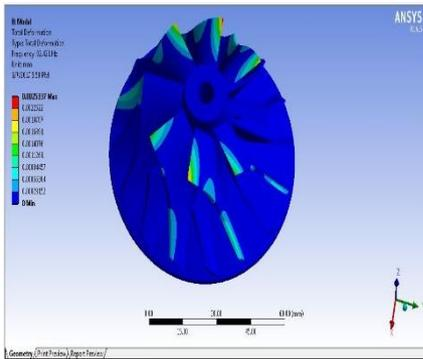
Mode shape 3 of Magnesium Alloy. At this mode the natural frequency of the impeller is 82.42Hz and deformation is 0.002533 mm.
