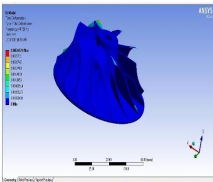
Mode shape 5 of Monel K500. At this mode the natural frequency of the impeller is 44.729Hz and deformation is 0.002667 mm.
