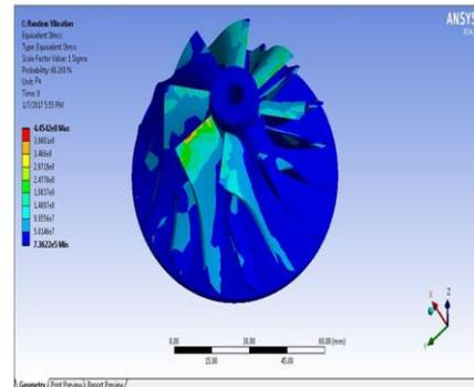
Stress induced in Magnesium Alloy Impeller in random vibrational analysis. The stress induced is 445.42 MPa
