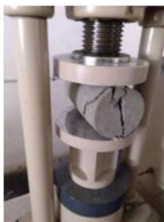
Figure :27- Split test of water proofing material curing specimen
