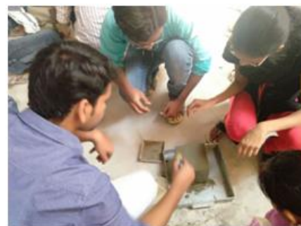
Fig:18-Application of water proofing material to the cube.
