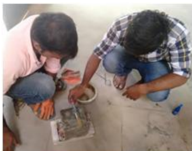
Fig 15: Applying of wax and after application of wax to the cubes
