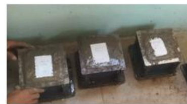
Fig casting of cubes
