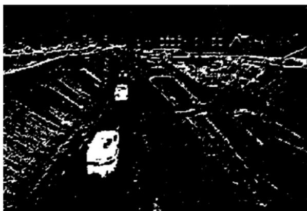
Fig. 7. Filtered result of Figure 3 by morphological close, ellipse type, size is 2x2.
