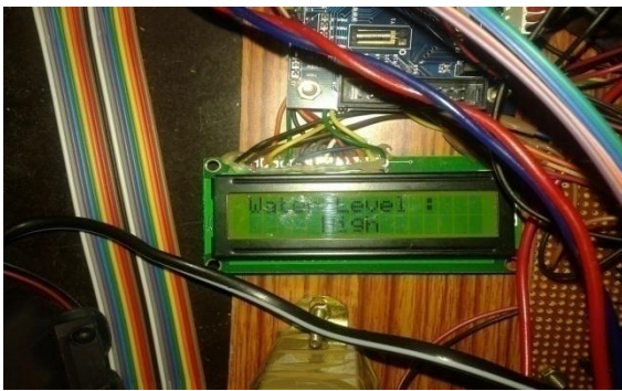
Fig-1: Image of the proposed model water level monitoring display on LCD
