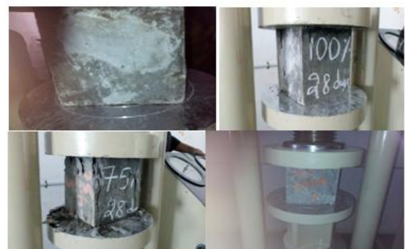
Compression testing of cubes
