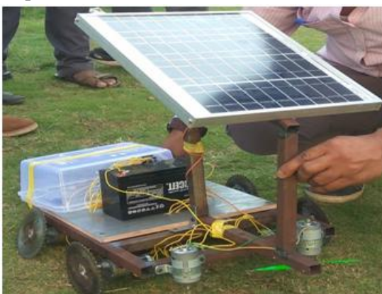
WORKIND MODEL OF AUTOMATED GRASS CUTTING AFTER ASSEMBLING ALL THE COMPONENTS
