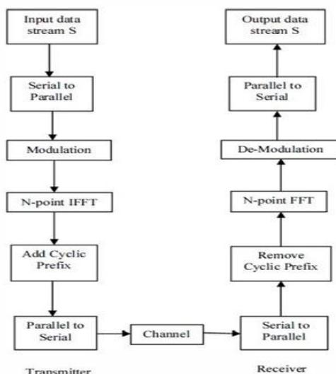
Figure 1: OFDMA System Model
