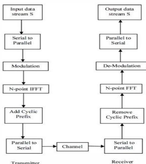
Figure 1: OFDMA System Model
