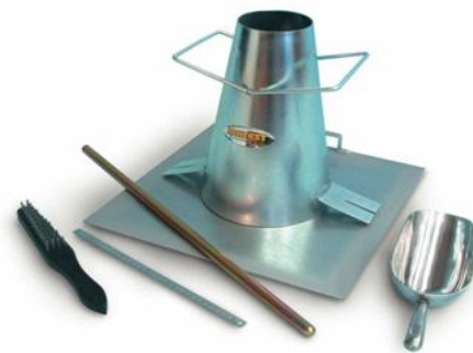
Fig 3.9 Slump Cone Apparatus
