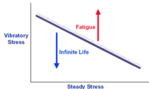
**Fig. 1.2 Advanced Airfoil Stress Range diagram**
