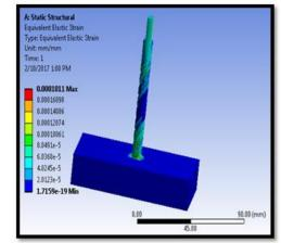
12mm DIAMETER - 118<sup>0</sup> ANGLE MATERIAL –ALUMINIUM FORCE – 900 N
