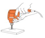
MODELS OF DRILLING TOOL AND WORKPIECE DIAMETER – 8mm 118<sup>0</sup> ANGLE CUT
