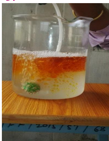
Dehydration is carried at 120°C and biodiesel is obtained
