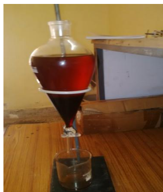
Separate the glycerin and oil wash the oil with water.
