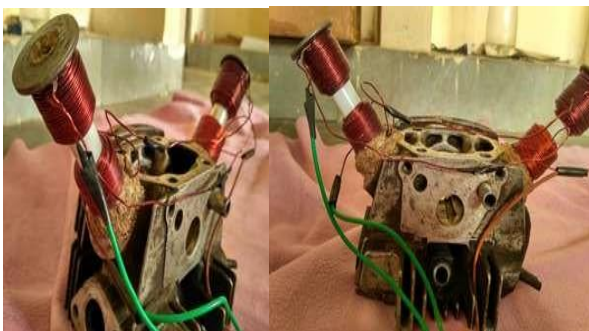
Fig.3.Side View and Front view of Solenoid Operated Camless Engine
