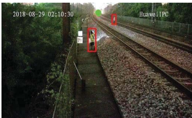
Fig. 1. A railway scene (1920*1080) contains intruding Foreign objects (red rectangle) and a vanishing point (green circle).
