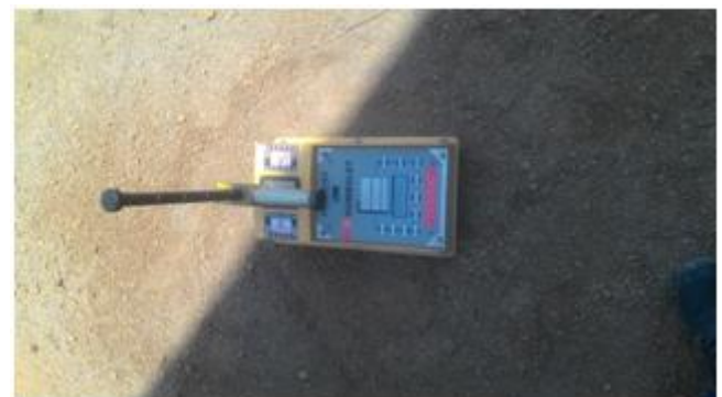
Fig.: NUCLEAR DENSITY GAUGE – used for in situ density measurement of soil
