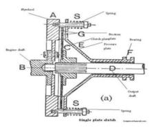
The facings and the waved cushion springs are riveted to a spring base disc and spring retainer plate. The waves of the cushion springs compress slightly as the clutch engages and thus provide some cushioning effect. The base disc and the spring retainer plate are slotted for inserting the torsion springs. These torsion springs contact the hub flange that fits between the spring retainer plate and the disc.
