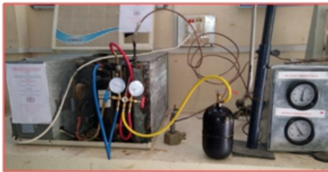
Fig 3.1 Experimental setup of air cooled condenser
