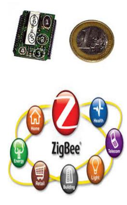
ZigBee module. The €1 coin, shown for size reference, is about 23 mm (0.9 inch) in diameter. ZigBee is a specification for a suite of high level communication protocols using small, low-power digital radios based on the IEEE 802.15.4-2003 standard for wireless personal area networks (WPANs), such as wireless headphones connecting with cell phones via short-range radio.
