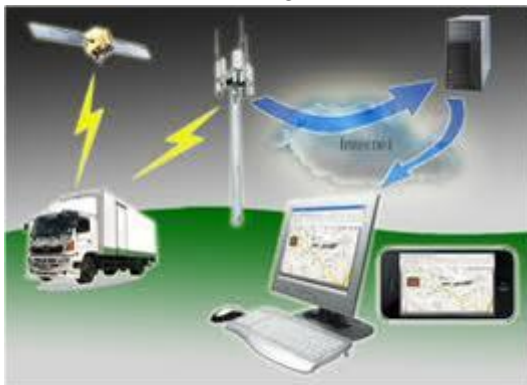
Fig 1: Positioning and monitoring system architecture
