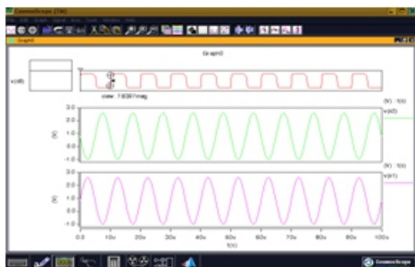
Fig 4(b).Output waveform of class AB two stage p-amps with current replicating branch using adoptive load II.
