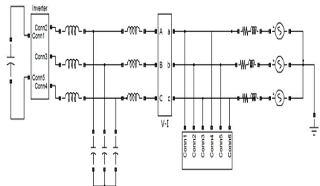
Fig 4: simulation design of the power system, including the STATCOM
