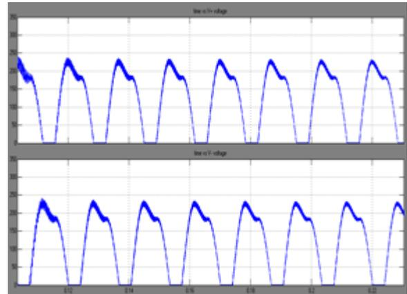
Fig 6: Simulation wave forms of  $V^+$  voltage loop and  $V^-$  voltage loop
