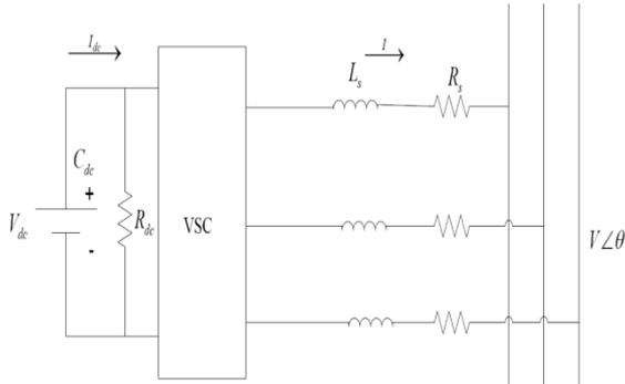
**Fig 1: STATCOM equivalent circuit**
