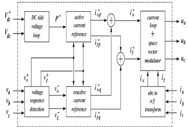
Fig 3: The STATCOM control system.
