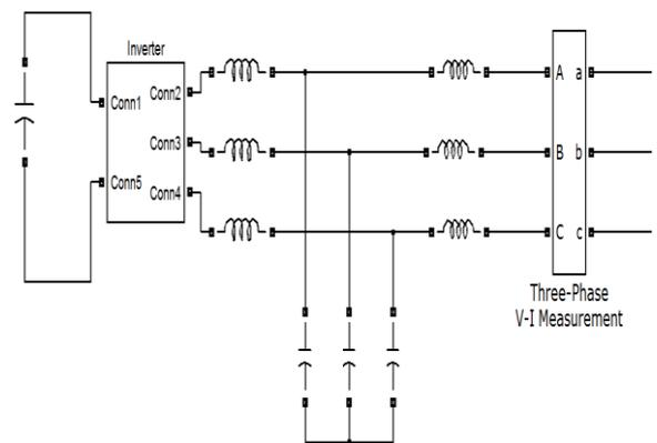
**Fig 2: simulation design of STATCOM**
