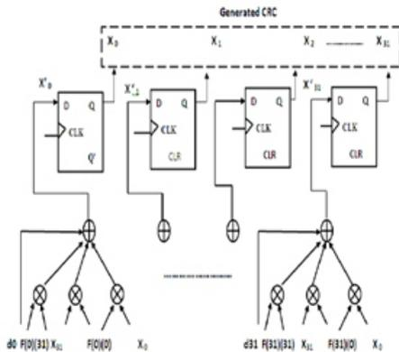
Fig: 5 Parallel Calculation CRC 32 for 32 bit
