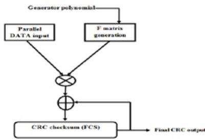
Fig: 4 Algorithms for F-matrix based Architecture
