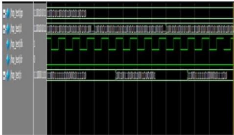
In proposed architecture  $d_i$  is the parallel input and  $F(i, j)$  is the element of  $F_{32}$  matrix located at  $i$ th row and  $j$ th column. As shown in figure 3 input data bits  $d_0 \dots d_{31}$  are ANDed with each row of FW matrix and result will be XORed. The proposed CRC-32 architecture with 64bit parallel bit simulated in Xilinx 9.2i ISE simulator. Input data bit to system is FFFFFFFFFFFFFFFF (64 bit).
