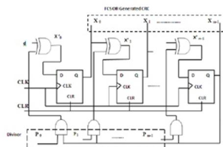
**Fig1. Basic LFSR Architecture**
