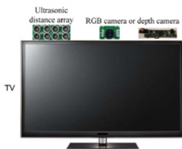
Fig. 1. The proposed TV control system's hardware components include the TV, set-top box, and some sensors, including the RGB or depth camera module and ultrasonic distance array module.
