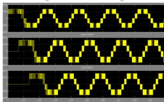
**Fig 14: Five-level inverter output voltages of three phases.**
