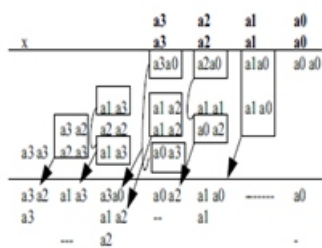
Fig.6. Partial product generation of 4x4 square unit
