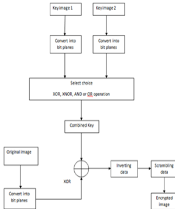
Fig.1 Proposed block diagram for Bitplane Crypt algorithm
