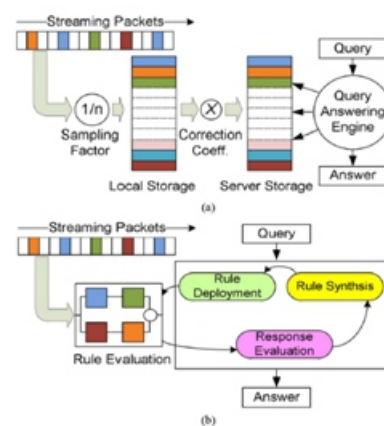
Fig. 1. Network measurement paradigms. (a) Traditional sampling-based methods. (b) Iterative measurement framework.
