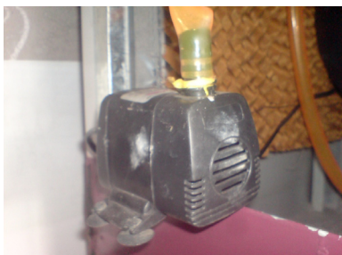
Figure 7: Image of Feed Pump
