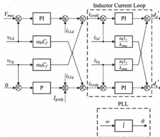
**Fig. 5. Simplified block diagram of the unified control strategy when DG operates in the islanded mode.**
