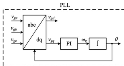
**Fig. 4. Simplified block diagram of the unified control strategy when DG operates in the grid-tied mode.**
