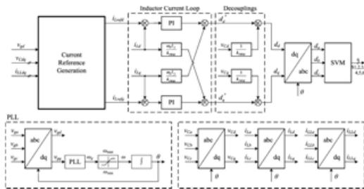
**Fig. 2. Overall block diagram of the proposed unified control strategy.**
