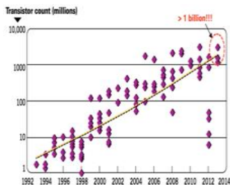
Figure 2.1. Evolution of transistor integration on a chip 3
