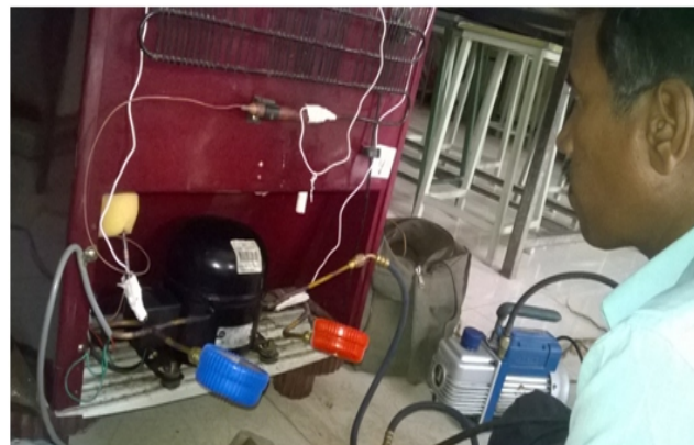
Figure 4.4: Refrigerator set up when Gas Charging of R134a
