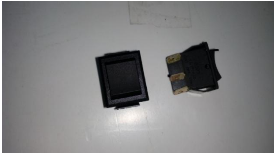
DPDT (double pole double through)
