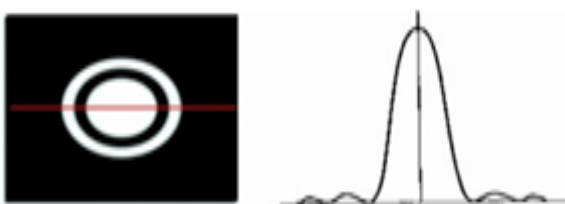
Fig 2.2 Point Spread Function (Airy Disk Pattern) of a point source
