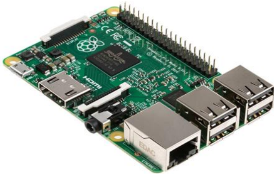
Figure-2: Raspberry Pi diagram
