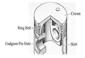
The major factor of difficulty in piston production is the CNC machining process. To obtain the desired clearance, the piston skirt should be machined with a tolerance of about  $\pm 0.004$ mm. This is because the piston must fit loosely enough to allow the piston to move, but tight enough that virtually no air or fluid in the cylinder can leak past it.
