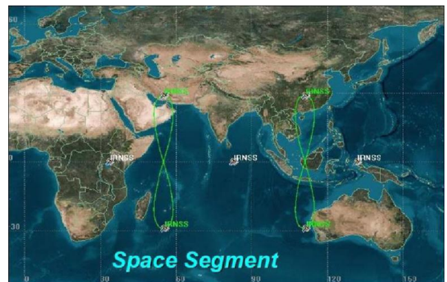
Figure 1: The IRNSS constellation with the daily lemniscates projection of the 4 GSO spacecraft onto Earth (image credit: ISRO)
