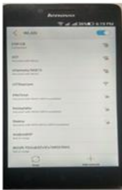
Fig 9 : Switch ON WI-FI And Select ESP-C8 Signal When Wi-fi is ON search & to select ESP-C8 signal and then the password is open door.
