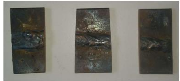
Fig 5: Welded MS plate after cutting
