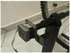
Electromagnetic damper (also called electromechanical brakes or EM brakes) slow or stop motion using electromagnetic force to apply mechanical resistance. The original name was "electromechanical brakes" but over the years the name changed to "electromagnetic brakes", referring to their actuation method. Since becoming popular in the mid-20th century
