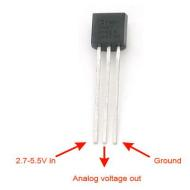
The Temperature Sensor LM35 sensors are precision integrated-circuit temperature sensors, whose output voltage is linearly proportional to the (Centigrade) temperature.
