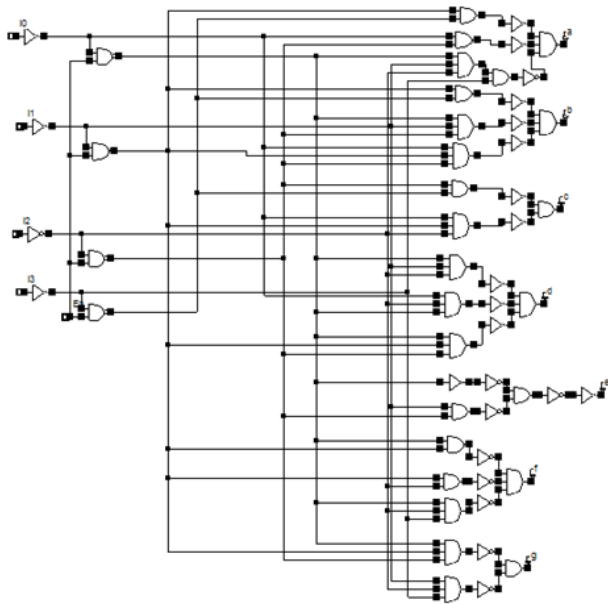
Figure 14. Schematic diagram of a 7-segments decoder
